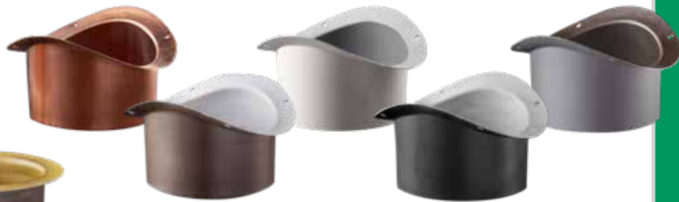
WIDE FLANGE HEAVY .032 HALF-ROUND OUTLETS 5/8" flange allows installation outside of gutter (more mechanically correct) if desired with holes for rivets or screws. Available in 3", 4" & 5" Copper and 4 Aluminum Colors: Dark Bronze, Low Gloss White, Black and Primer Grey
