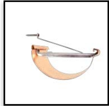
Clip and Screw with tie strap is fascia mounted. Tie Strap is stainless steel and the bracket is available in 5", 6" & 8" aluminum and stainless steel
